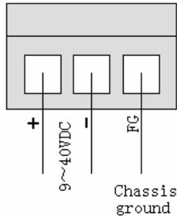
Wiring diagram of power terminal
