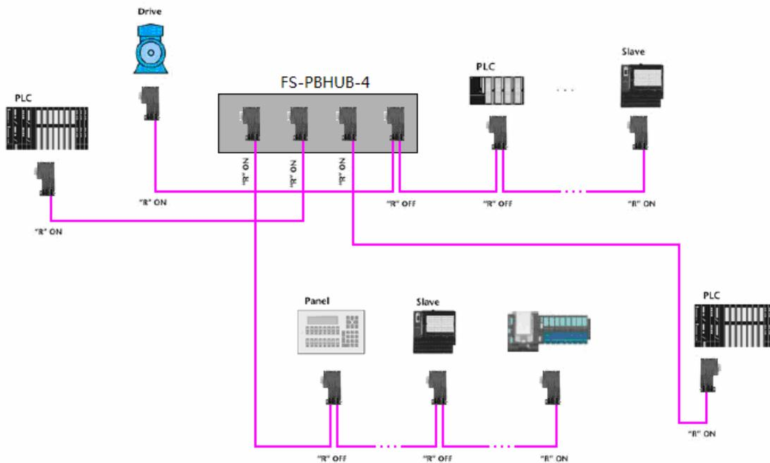
Fig.6-2 Hybrid network topological structure through FS-PBHUB-4
