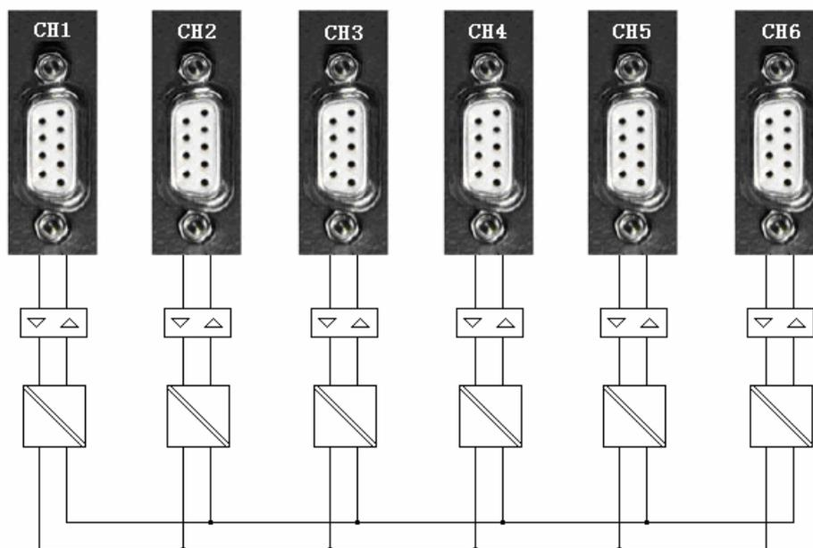
Fig. 5-1 Internal Functional Block Diagram of PROFIBUS Hub
