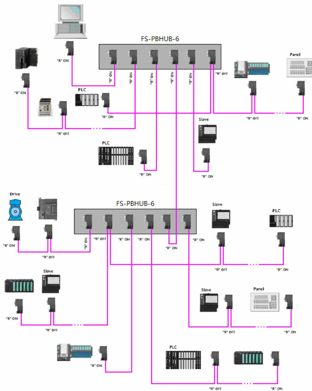
Fig.6-3 Hybrid network topological structure through FS-PBHUB-6
