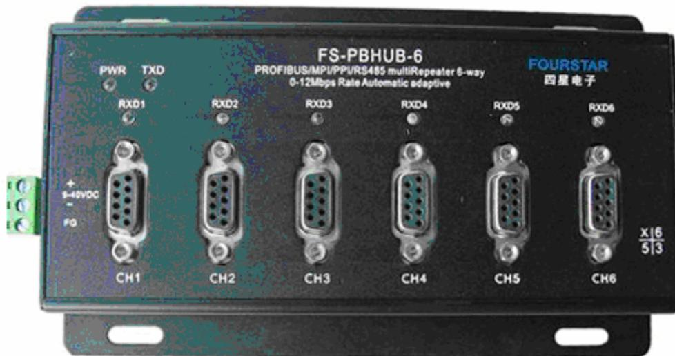
Fig. 4-1 Outline Drawing of Fourstar FS-PBHUB-4 and FS-PBHUB-6
