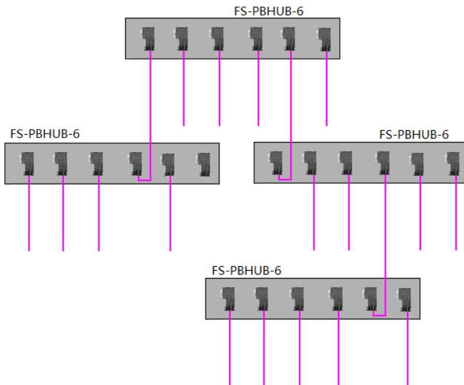
Fig. 2-2 Cascade connection of PROFIBUS Hub
