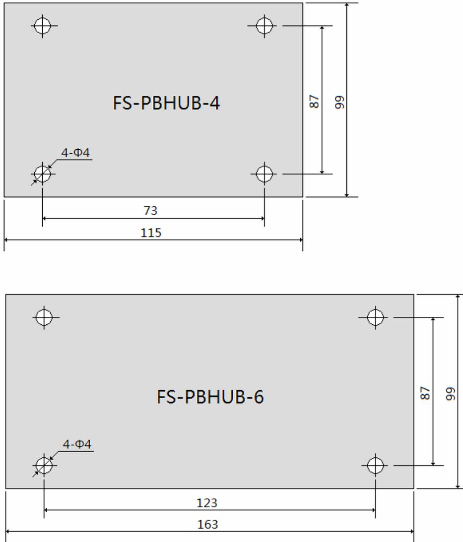
Fig. 4-2 Mounting Size Drawing of Fourstar FS-PBHUB-4 and FS-PBHUB-6
