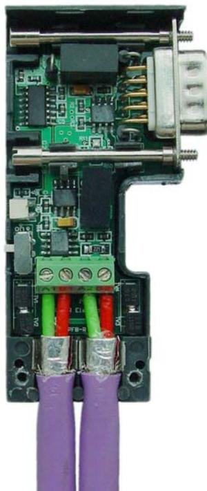
3. Indication light: An emitting diode indication light exists on PFB-R. When A2 & B2 of RS485 send data to the bus cable, the indication light blinks at 5Hz.
