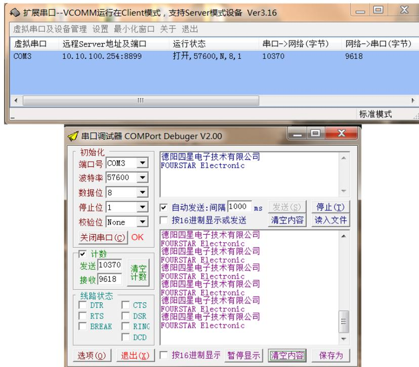
Figure 11-1 Screenshot of virtual serial port software and serial port testing software
