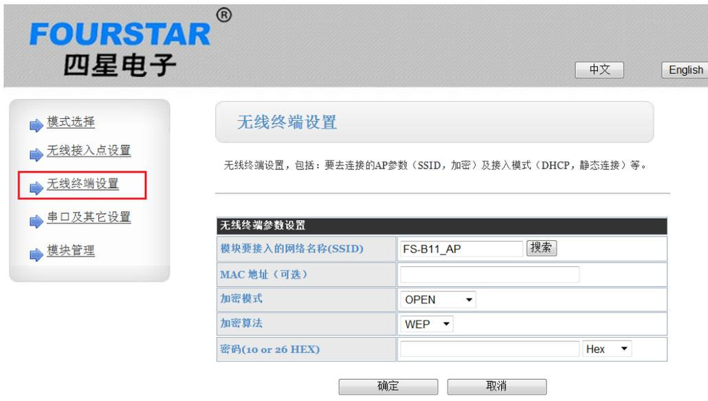
Figure 4-4 Setting of wireless terminal (Station)
