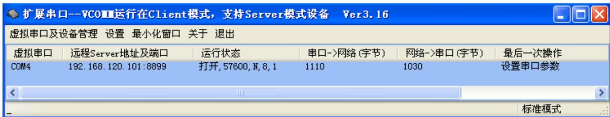
Figure 10-10 Operation state of virtual serial port software
