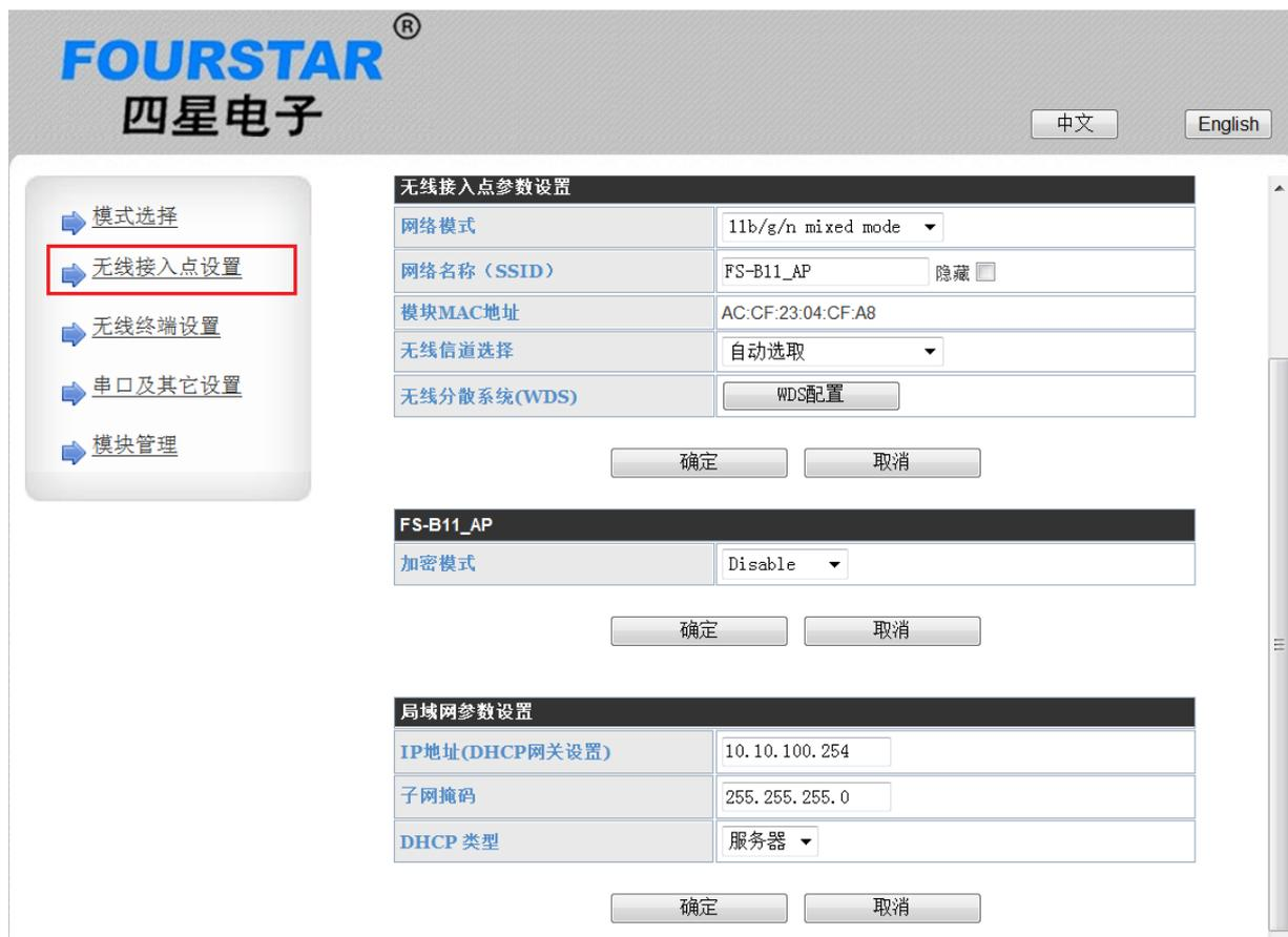
Figure 4-3 Setting of wireless access point AP
