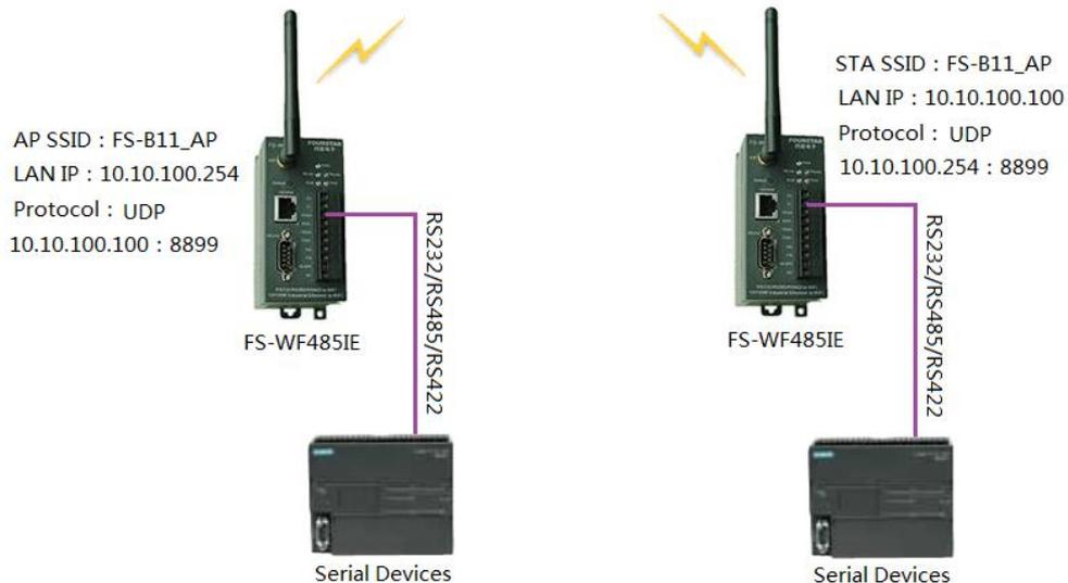
Figure 6-4 UDP unicast point-to-point connection
