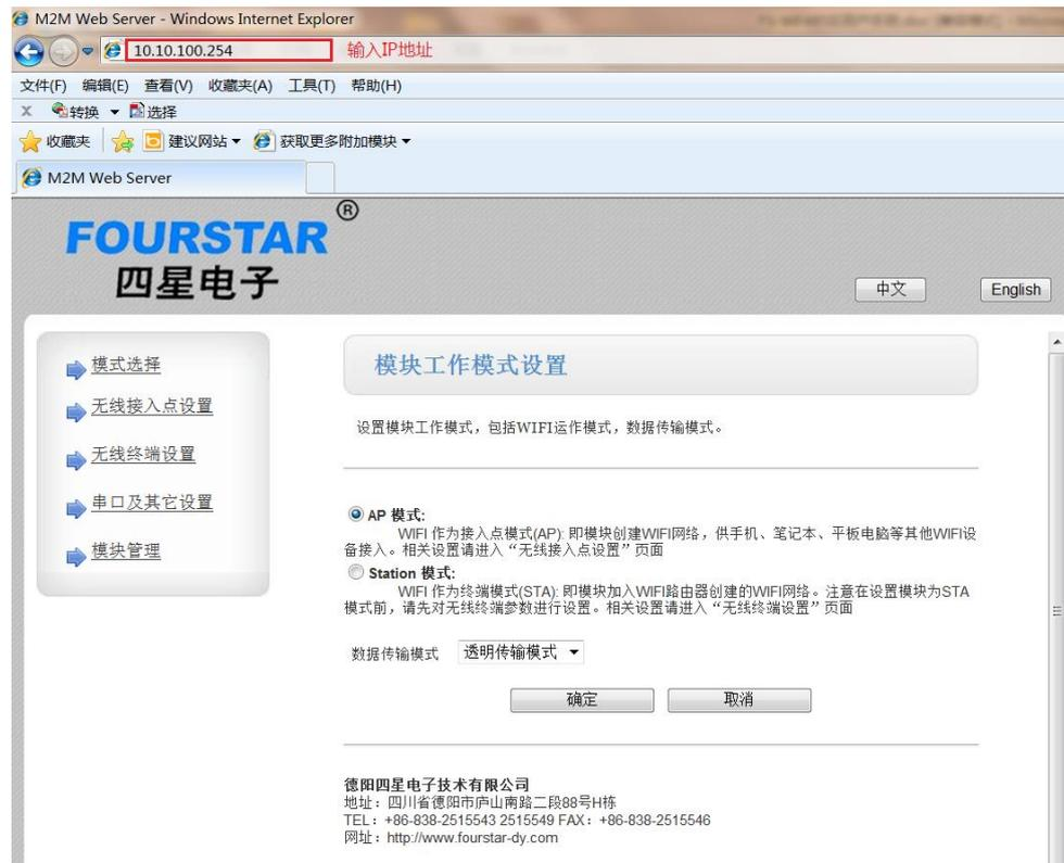
Figure 4-2 Web setting interface of FS-WF485IE
