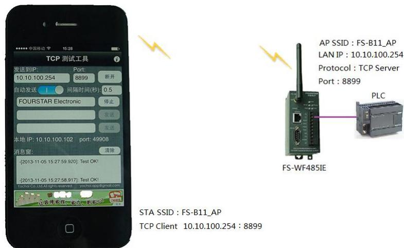
Figure 8-1 Communication between mobile phone and FS-WF485IE
