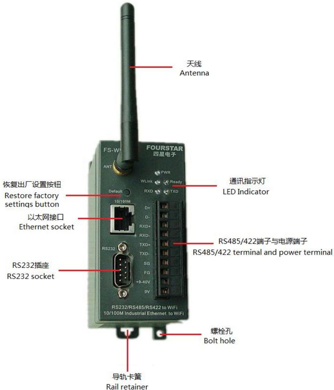
Figure 3-1 External structure and description of parts for FS-WF485IE
