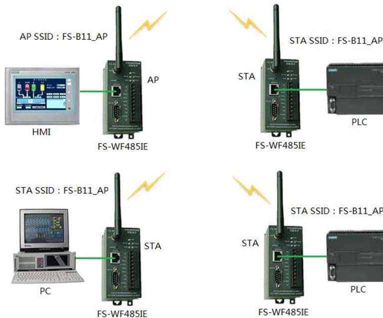
Figure 5-2 Network topology for Ethernet to wireless WiFi
