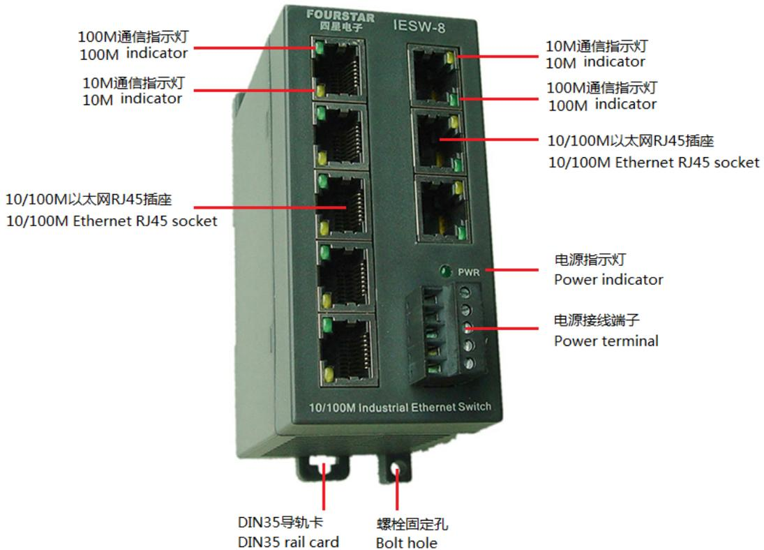
Fig.3-1 Diagram of External Structure of IESW-8
