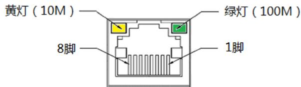
Fig.3-2 RJ45 Socket of Ethernet
